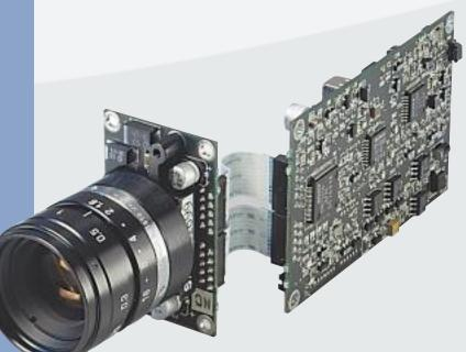
Asynchronous reset accepts an external trigger input to reset the camera to the beginning of the vertical interval (field 1, line 1). The first field of video information reads out 9.5 horizontal lines after triggering.
